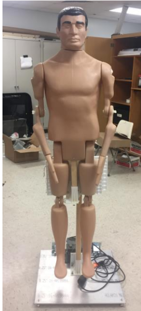
Figure 5: Ready-to-Fall position and stand to dummy interface.
